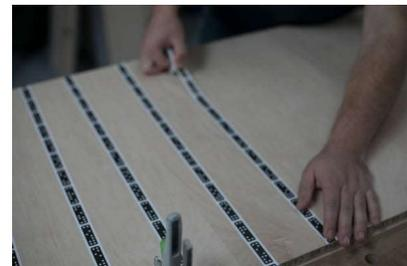
We find that laying ShaperTape out in roughly parallel lines is easiest, but there is no need to be precious about this, as the strips do not need to be exactly parallel or exactly uniform in length. The orientation of tape in reference to your workpiece (parallel/perpendicular/diagonal) is not critical, and should be adapted to suit your project. However, no tape should overlap.
